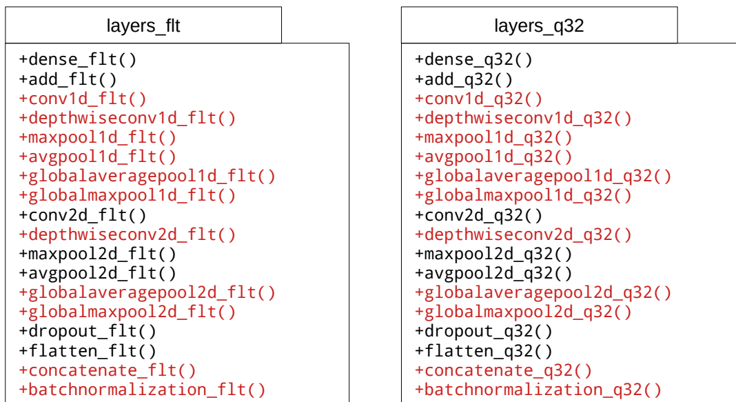
Figure 29: Emmi Core modules layersflt and layersq32
