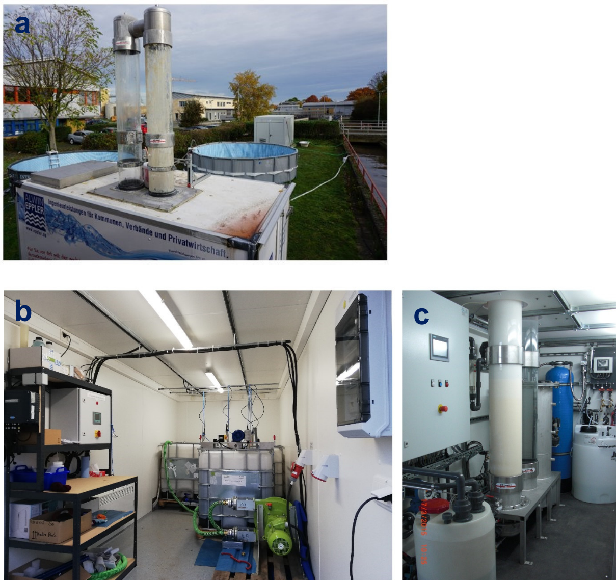
Figure S5-5 | Re-BioP-Cycle pilot plant for P recovery built at the municipal WWTP Giessen. a) Overview; front: precipitation unit; middle: storage tank unit B; back: 20 ft container with the P re-dissolution reactors. b) P re-dissolution unit A. c) precipitation unit C designed by ALWIN Eppler GmbH & Co. KG.
